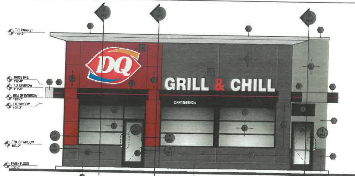
1 FRONT ELEVATION A3.1 SCALE: 1/4" = 1'-0" NOTE: THE DQ RED SPOON HANDLES HAVE SPECIAL INSTALLATION REQUIREMENTS. ALUM. STOREFRONT MFG. MUST COORD. LOCK & HANDLE, LOCATION & HEIGHTS
